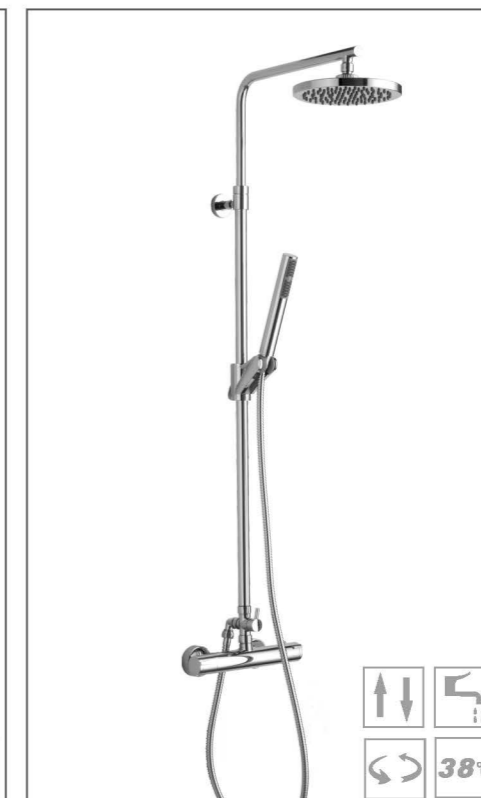
HL-3120 Material:Brass(Φ19-24mm) Size:(1000-1300)X550X200mm Rain shower:HL630ABS(Φ200mm,ABS) Hand shower:1F1818H(1Function,ABS)
