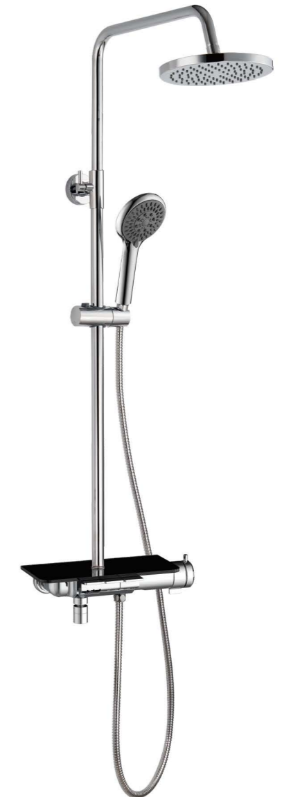
HL3831G Material: Stainless Steel 304 tube(Φ24mm) & Brass Mixer Size: 1000~1300x300x450mm Rain shower: 1F660ABS ( Φ200mm, ABS) Hand shower:5F8001, Φ100mm, ABS)
