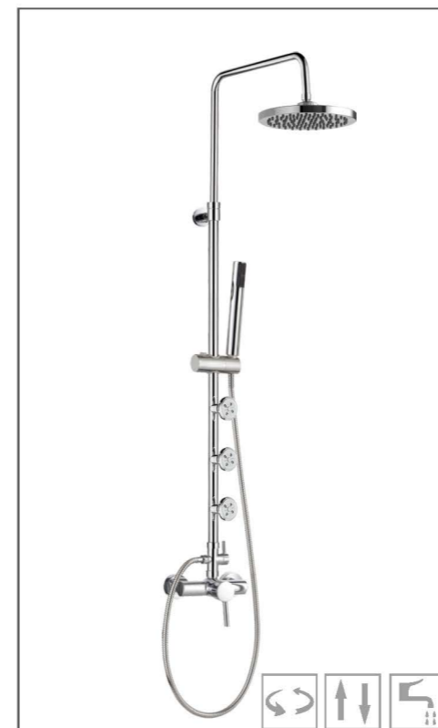
HL-3308 Material:Brass(Φ19-24mm) Size:(1000-1300)X550X200mm Rain shower:HL630ABS(Φ200mm,ABS) Hand shower:1F1818-30(1Function,ABS)
